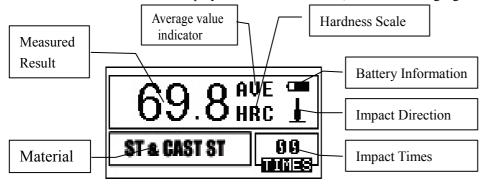
The measured values are displayed with big font in this interface, and multiple shortcut key operation functions supplied.
