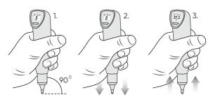
Sudden pressing or shifting of the probe is not allowed – this may lead to exceeding the permissible error margin and cause chipping of the diamond indenter.
